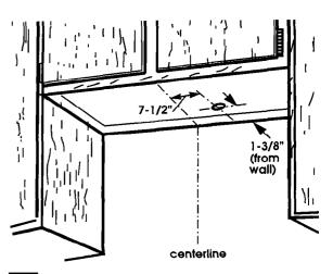
To wire through top, mark a line 7-1/2" from the right of the centerline on the underside of the cabinet. Mark the point on this line that is 1-3/8" from the back wall. Drill a 1-1/4" diameter hole through cabinet at this point.
